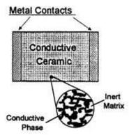
The simple construction, consisting mainly of the conductive ceramic material with bonded metal contacts, is highly reliable. Selection of the proper material from among several options allows the properties to be controlled and tailored to the application.
