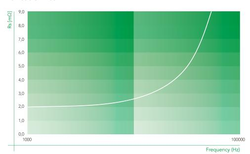
Typical DCH85C Series Resistance at ambient temperature for a specific model. For the characterization of a different model, please contact R&D department.
