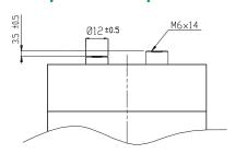
Two different terminals height for special BUS BAR coupling.
