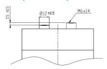
Two different terminals height for special BUS BAR coupling.
