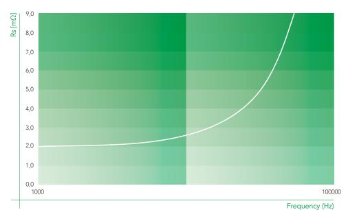
Typical DC 85C Series Resistance at ambient temperature for a specific model. For the characterization of a different model, please contact R&D department.
