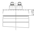
Dimension with overpressure device activated
